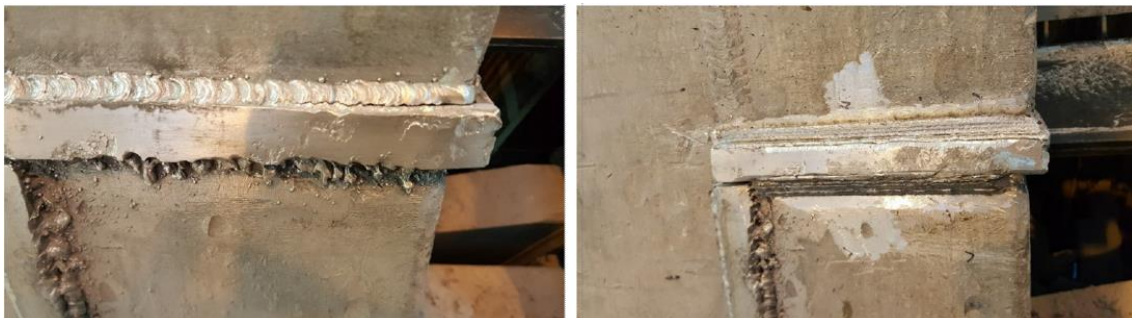
Figure 4. Usual anode riser welding (left) vs laser welding (right).
