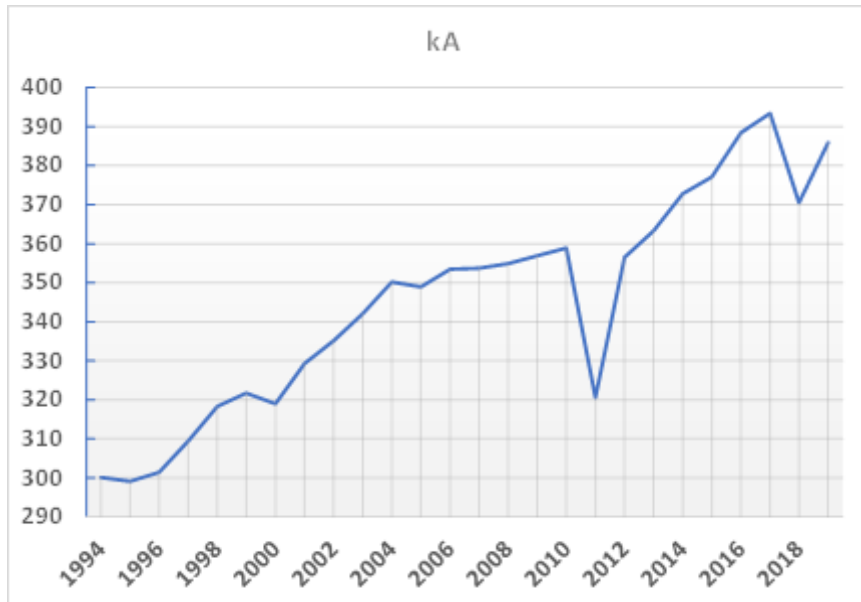
Figure 1. Amperage increase in Aluminium Dunkerque.
